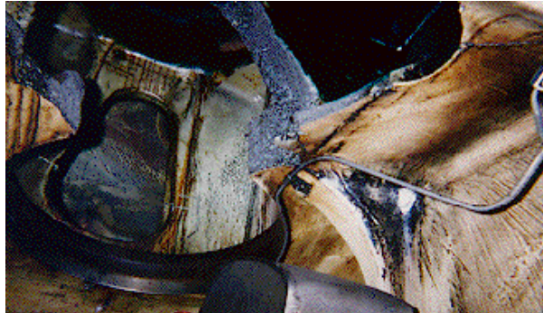
Cracked sleeve seat area.
